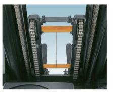
Three-stage mast with four-cylinder mechanism
